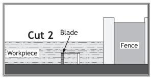
**Figure 53.** Second cut for a single dado cut.
